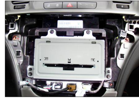
7. Remove OEM cd/radio parts
