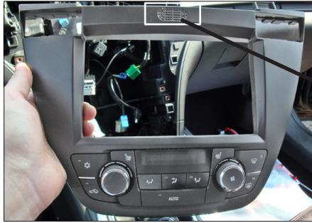
11. Mount air condition control unit to double DIN fascia place
