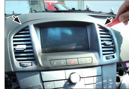
5. Unclip and remove OEM display
