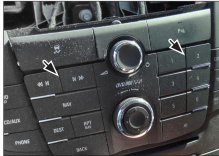
12. Remove switch for ESP (left) and switch for Park Distance Control (right). Put them to the openings at the top of double DIN fascia plate.
