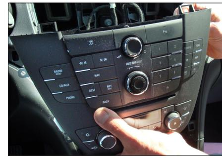
6. Unclip and remove OEM head unit
