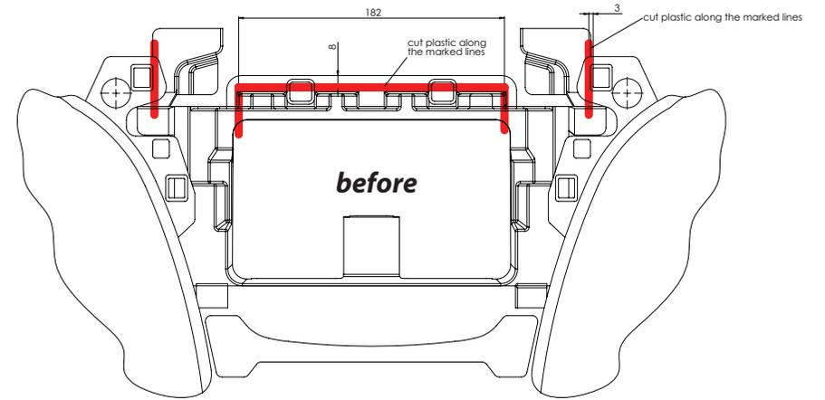
10. Cut plastic from dash board in order to clear space for the double DIN head unit (see lines in the drawing)
