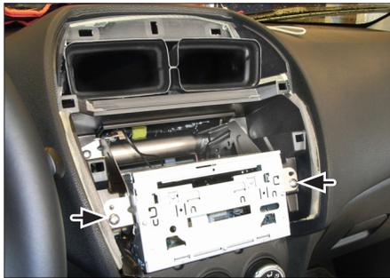
2. Remove OEM Radio/CD device
