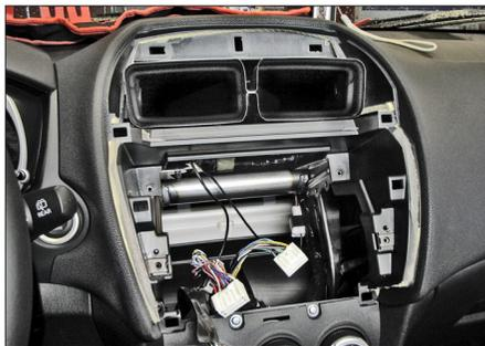
3. Dashboard with removed OEM Radio/CD device
