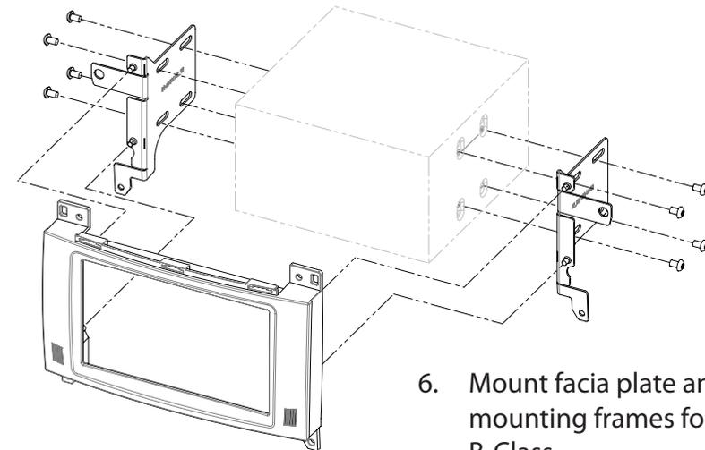
6. Mount fascia plate and mounting frames for A-Class / B-Class
