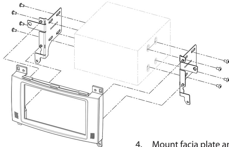
4. Mount fascia plate and mounting frames to double DIN head unit
