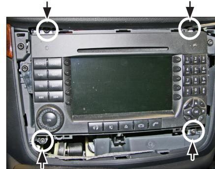
2. Remove the four screws at the top and bottom of OEM head unit.
