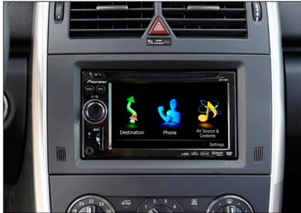
7. Connect all required circuit points and push double DIN head into dash board
