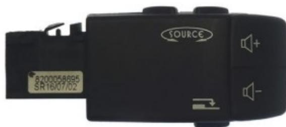
The interface can also be used with the older stalk paddle pictured above. The left SOURCE button will change the source, and the right SOURCE button will work as the phone answer/reject button. Short press to answer a call, long press to reject.
