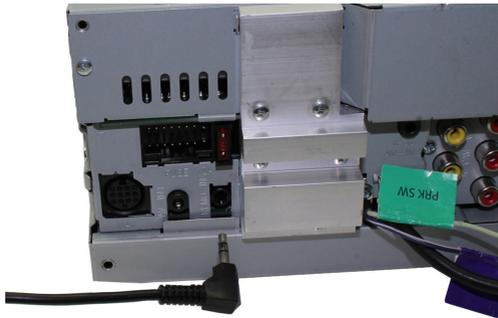
4. Select the correct harness (8-way ISO or Quadlock) for your vehicle. Connect the 14 way molex connector to the interface
