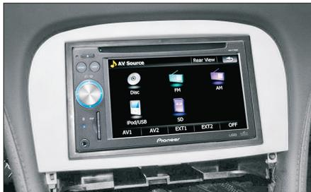
7. Connect all required circuit points to the head unit and push it into the metal frame until it snaps in. Place the trim frame.
