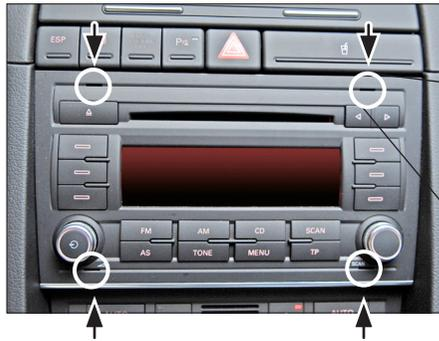
1. Put four radio release keys in the appropriate slots of the OEM radio
