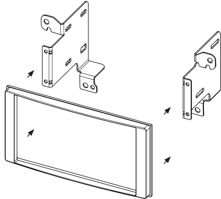
4. Slide double DIN head unit into the brackets/facia plate and secure to the assembly with screws
