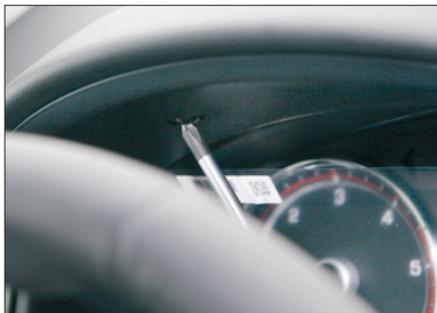
4. Remove 2 screws beneath tachometer unit cover left and right side
