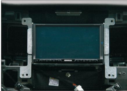
9. Attach metal mounting brackets to Double-DIN navigation
