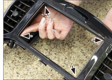
6. Attach facia plate to OEM panel using Glue
