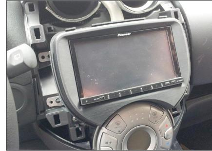
5. Mount mounting frames to double DIN head unit
