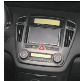
5. Connect all required circuit points to the head unit and push it into the metal frame until it snaps in. Place the facia plate.
