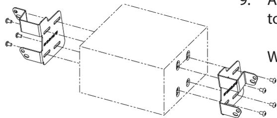
9. Attach mounting brackets to 2-DIN head unit
