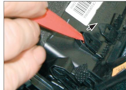
7. Unclip and remove air vents
