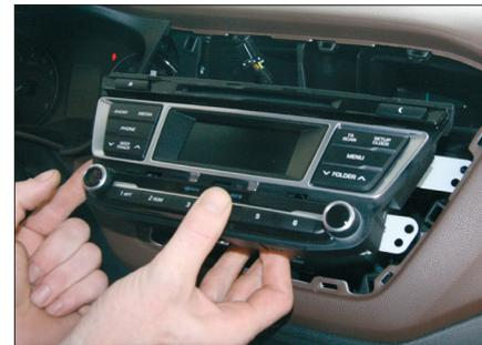
8. Remove OEM head unit (unplug all cables carefully)
