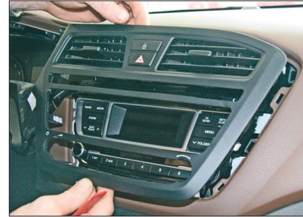
5. Remove OEM center panel (unplug cables carefully)
