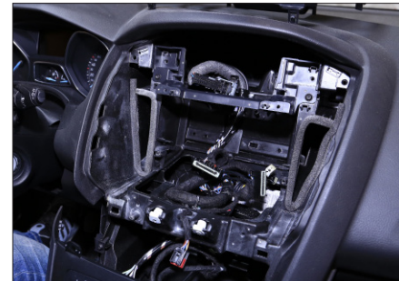
6. Remove OEM center panel
