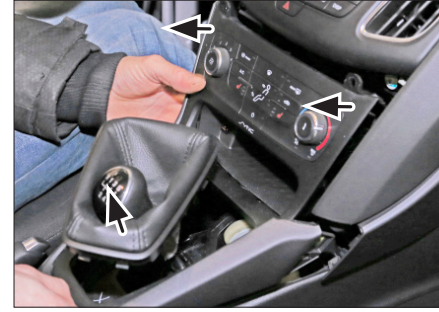
5. Unclip panels Unclip gear shift cover
