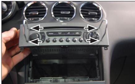
3. Insert two radio release keys in the openings of the OEM head unit.
