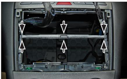
4. Remove middle bar to clear space for the Double DIN head unit.
