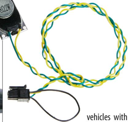
vehicles with 4 line dash display only: Cut and insulate this (black) loop
