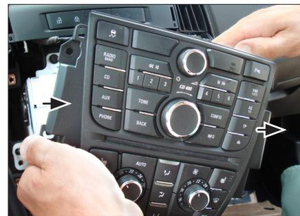
6. Remove screws of OEM control unit
