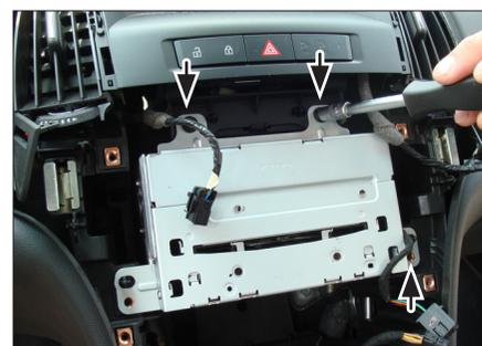
7. Remove screws of OEM head unit
