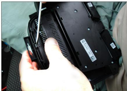
10. Unclip air condition control unit from OEM panel
