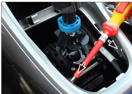
2. Remove screws of OEM center panel
