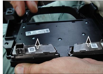
12. Remove switch left and switch right from OEM unit
