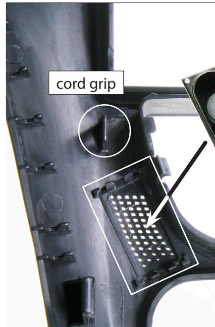
14. Connect speaker\* plug to steering wheel interface. Mount speaker to fascia plate. *Use cord grip for securing speaker cable*
