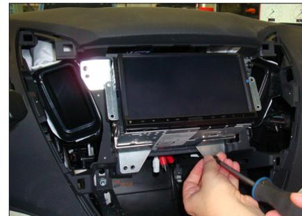
7. Mount mounting frames to double DIN head unit
