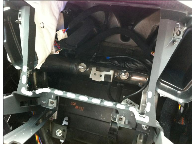
6. cut away here (see lines) to clear space for double DIN head unit
