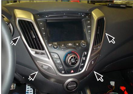
1. Unclip OEM panel with air vents (see arrows)
