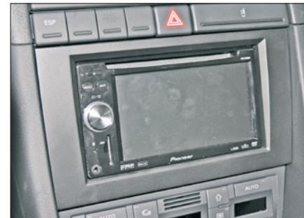
5. Connect all required circuit points and push the double DIN head unit in the metal frame until it snaps in.
