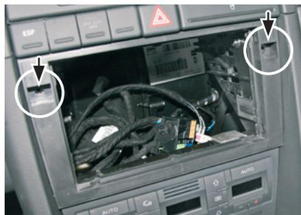
4. Fix the mounting frame with two screws (see arrows)
