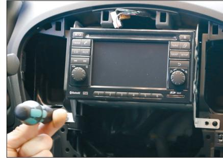
5. Remove screws of OEM
