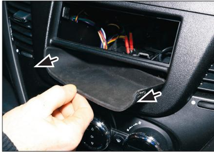
2. Remove anti-slip mat (fixed with double-sided tape)
