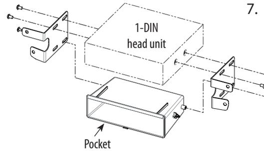
7. 1-DIN + pocket: Mount brackets with distance of ~ 11 mm to unit front surface
