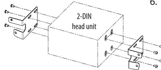
6. 2-DIN: Mount brackets with ~ 19 mm distance to unit front surface
