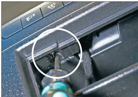
4. Remove 2 screws under to top side of the OEM panel (see arrows)
