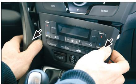
2. Remove air condition control panel (below the radio)
