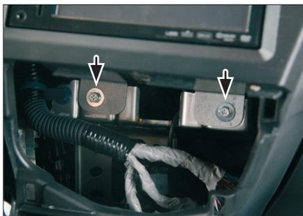
1. Connect all required circuit points push double DIN head unit into dashboard.
