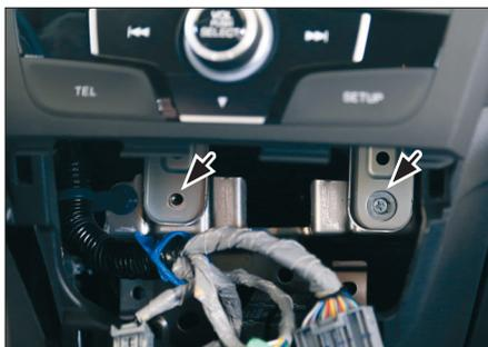
3. Remove both screws (keep screws, they will be needed later)
