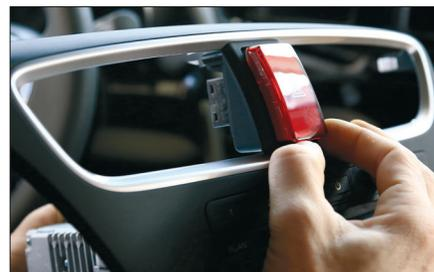
6. Remove hazard light switch from OEM panel
