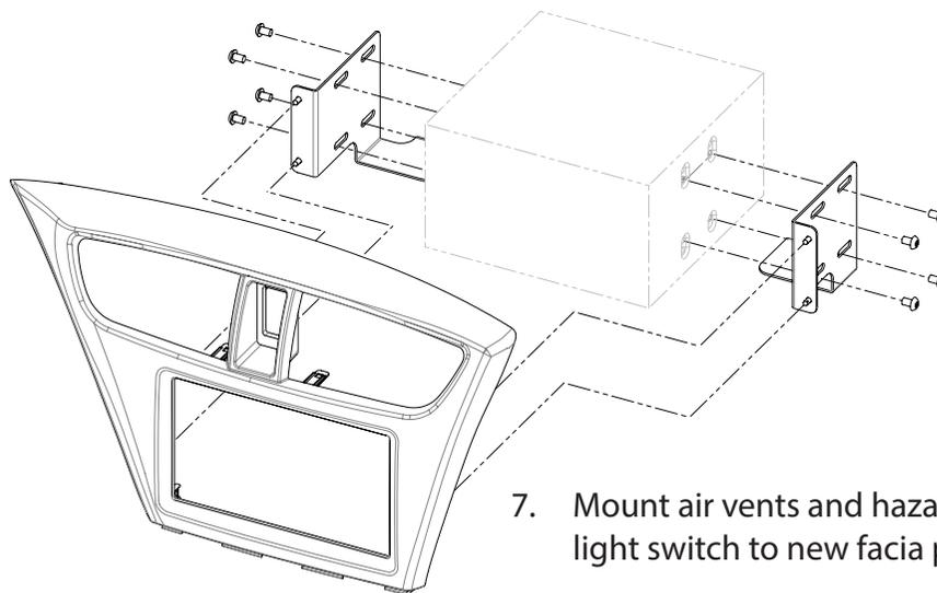
7. Mount air vents and hazard light switch to new facia plate
