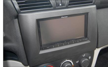
3. Connect all required circuit points and push the double DIN head unit in the metal frame until it snaps in.
