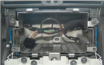
3. Remove two screws of the OEM metal frame (see arrows) at the left and right side.
