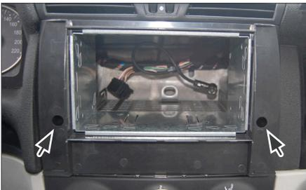
4. Push the metal frame into the mounting frame.
