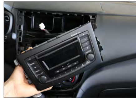
7. Unclip all connectors Remove OEM head unit
