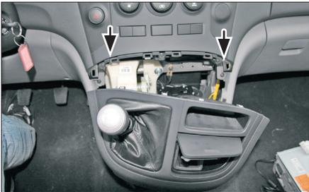
2. Unclip the gear lever box
