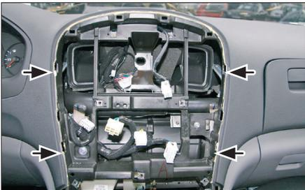
3. Unclip the front panel and remove it
