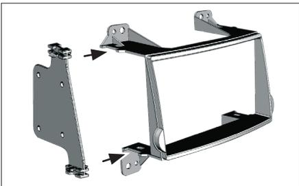
4. Attach the mounting brackets to the facia plate (see arrows)
