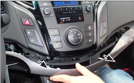
3. Unclip OEM bar under head unit (see arrows)
