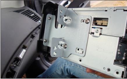
9. Attach mounting frames and facia plate to double DIN navigation
